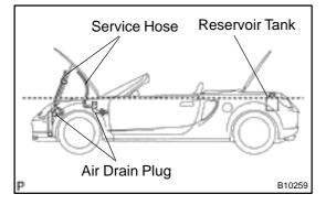
(5) Check with your eyes that the water level of the air drain service hoses of radiator and heater water valve is as high as that of the reservoir tank.
